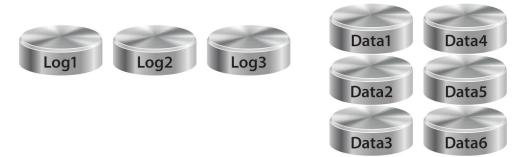
The figure above shows an example of a simplified Oracle data layout using a small number of equal-sized large LUNs for data, and one separate LUN for each of the redo log groups. In this example, a single Oracle data disk group using Oracle ASM can be created with the six larger LUNs, while three individual Oracle ASM disk groups can be created from the three smaller LUNs.
